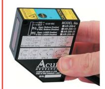
The AR200 family of triangulating laser displacement sensors has four models to satisfy your range requirements with excellent resolution and sensitivity. The most accurate model measures distances over 6 mm with a resolution of 2  $\mu$ m. The longest range AR200 sensor measures to 50mm with a resolution of 15  $\mu$ m.
